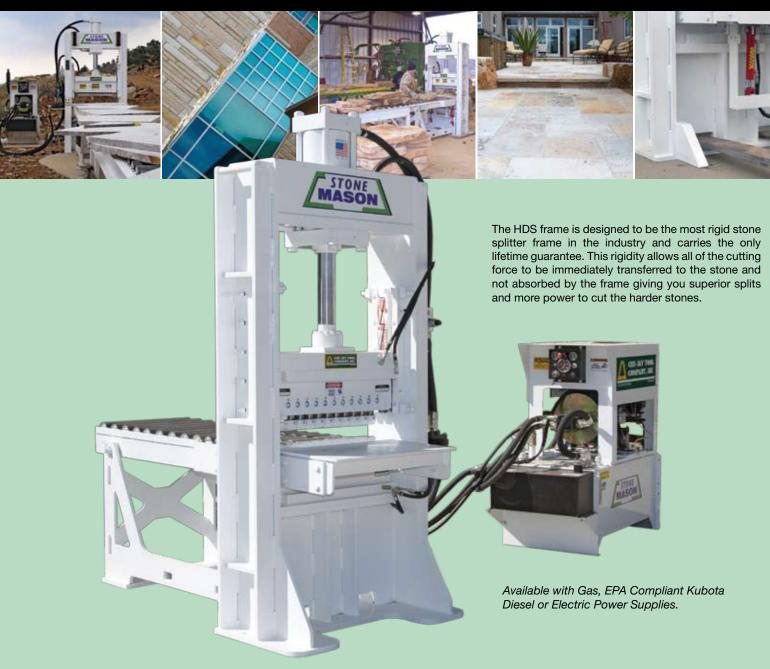
The **HDS** is a very tough and versatile production machine for splitting building stone or preparing stone for thin veneer sawing and is ideal as a compliment larger machine to split medium size boulders in a production line. The HDS has 26-inches of cutting teeth with a 32-inch wide and 16-inch high opening.
